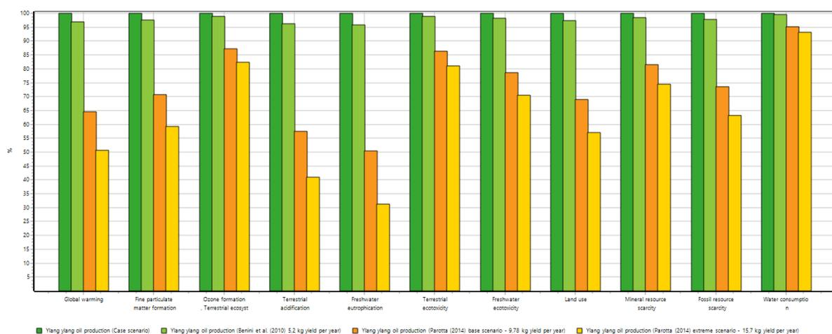
Figure 16 : ReCiPe 2016 Impact Comparison for yield. Case scenario: dark green; Benini et al. scenario: light green; Parotta base scenario: orange; Parotta extreme scenario: yellow. Categories follow the same order that they are presented in the Impact Assessment Methodology.
