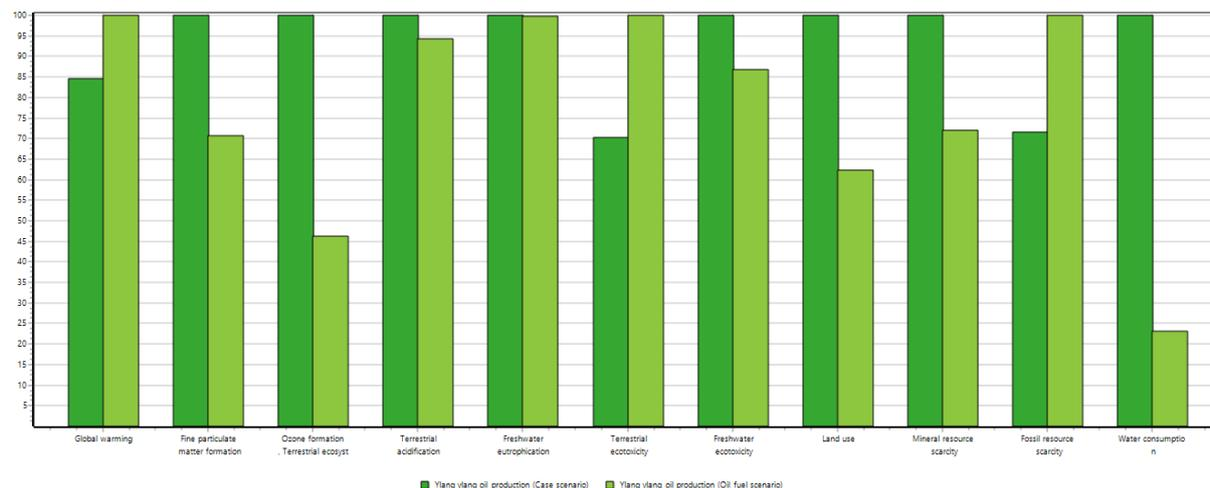
Figure 18 : ReCiPe 2016 Midpoint Impact Comparison for fuel. Case scenario (wood fuel): dark green; Oil fuel scenario: light green. Categories follow the same order that they are presented in the Impact Assessment Methodology.
