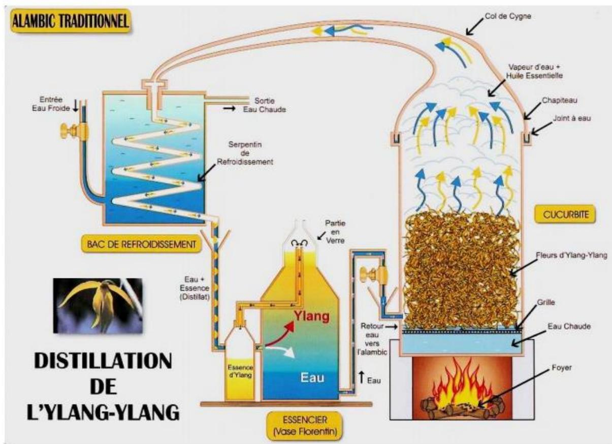
Figure 25: Another illustration of a traditional steam-distillation alembic system. Retrieved from de Bontin (2006).
