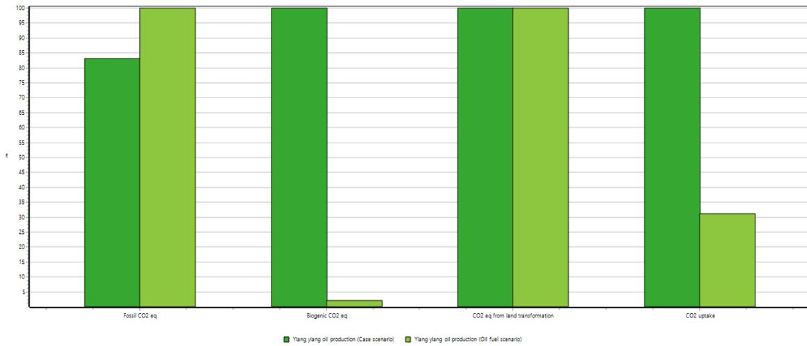
Figure 19 : GHG Protocol Impact Comparison for fuel. Case scenario (wood fuel): dark green; Oil fuel scenario: light green. Categories from left to right: Fossil CO2 eq, Biogenic CO2 eq, CO2 eq from land transformation, CO2 eq uptake.
