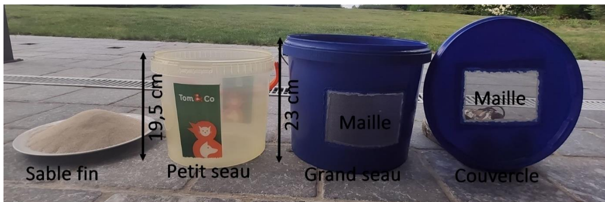
Figure 13 : Constitutants du Bucket in a Bucket
